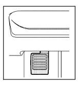
To set the parking brake, push down the parking brake pedal with your left foot. If the ignition is on, the brake system warning light will come on. See *Brake System Warning Light on page 207*.
